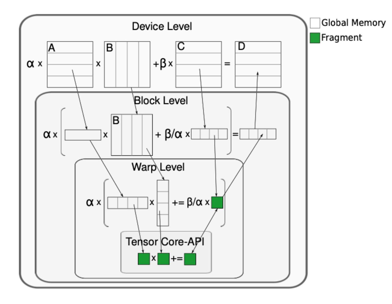
• CUDA offers a warp-level API for exploiting Tensor Cores
